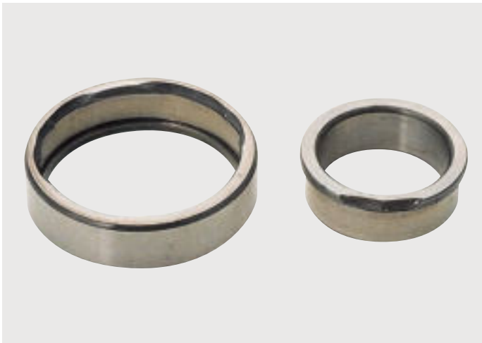
Photo C-1 · Cylindrical roller bearings · Chipping of inner/outer ring shoulder · Caused by excessive impact load
