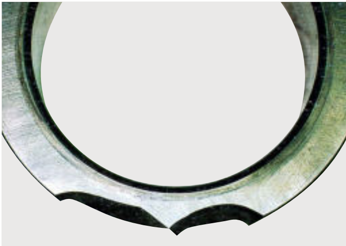
Photo C-3 · Tapered roller bearing inner ring · Extensive chipping of shoulder · Caused by impact due to poor assembly
