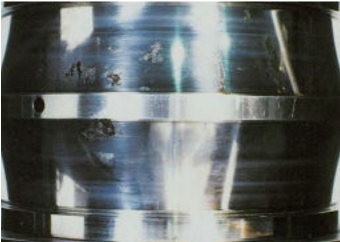
Photo D-4 · Spherical roller bearing inner ring (split type) · Rust and corrosion have occurred on surfaces of the raceway · Caused by water contamination
