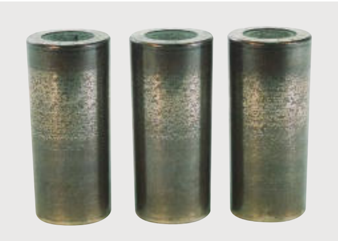
Photo B-3 · Tapered roller bearing rollers · Indentation has occurred on the rolling surface (temperature discoloration at both ends) · Caused by intrusion of foreign material in the lubricant
