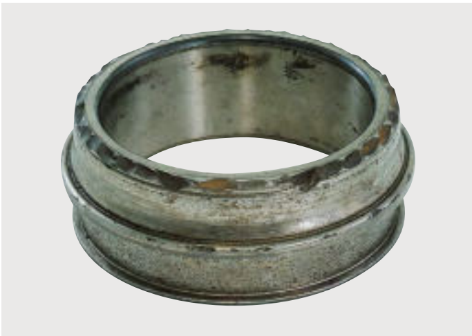
Photo C-2 · Spherical roller bearing inner ring · Chipping of shoulder section · Caused by excessive impact load
