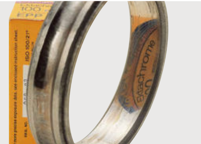
Photo G-1 · Deep groove ball bearing inner ring · Surface rust due to bore surface creep
