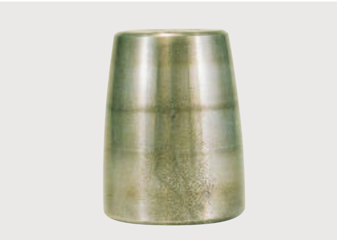
Photo D-3 · Spherical roller bearing rollers · Rust and corrosion have occurred on surfaces of the rolling surface · Caused by water contamination
