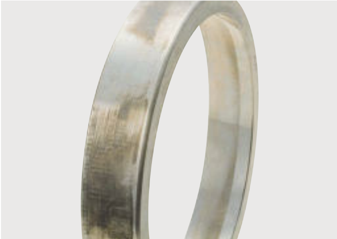
Photo F-4 · Tapered roller bearing outer ring · Fretting corrosion has occurred along the outer diameter
