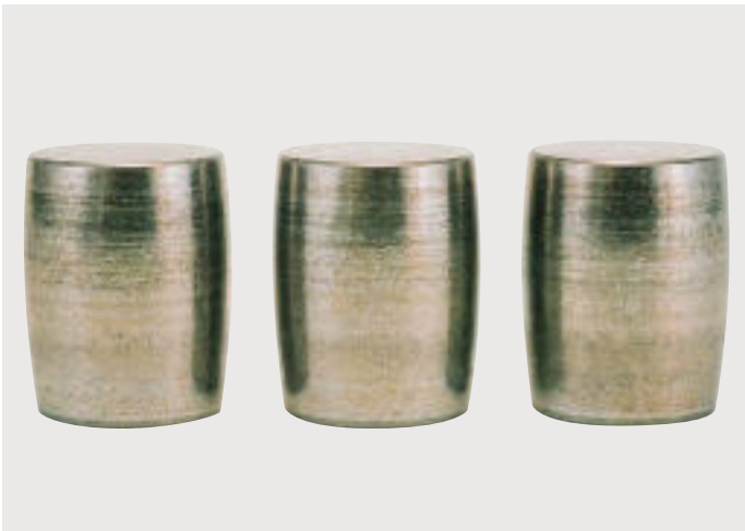
Photo B-2 · Spherical roller bearing rollers · Indentation has occurred on the rolling surface · Caused by compaction of solid foreign material
