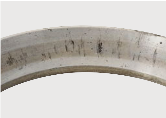
Photo D-2 · Tapered roller bearing outer ring · Rust formed at the pitch of the rollers on the raceway surface.
