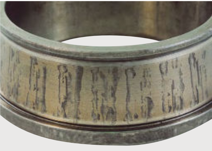
Photo D-1 · Tapered roller bearing inner ring · Rust formed at the pitch of the rollers on the raceway surface.
