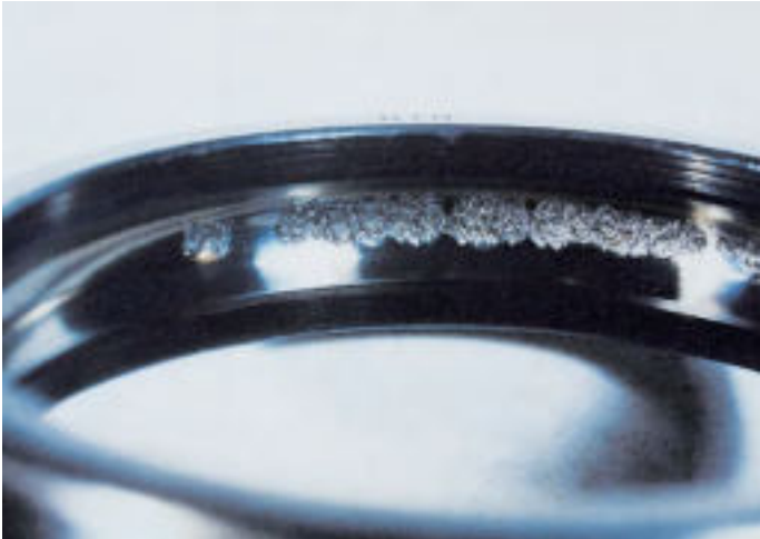
Photo A-2 · Angular bearing outer ring · Flaking caused by the ball pitch on the raceway surface · Caused by poor bearing handling
