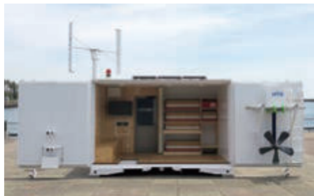
Example of assembled products application (fully equipped with a wind turbine, hydro turbine, solar panels, and storage batteries)
