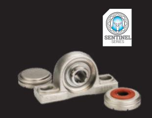
Stainless steel is generally more brittle than traditional 52100 bearing steel. Because of this fact, tightening inner ring set screws in stainless steel insert bearings with the proper torque is essential to avoid fracturing of the inner ring.
